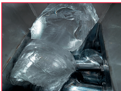
Processing of highly viscous base polymers such as butyl rubber and polyisobutylene (PIB) Tattamento di polimeri di base altamente viscosi come la gomma butile e il polisobutilene (PIB)
