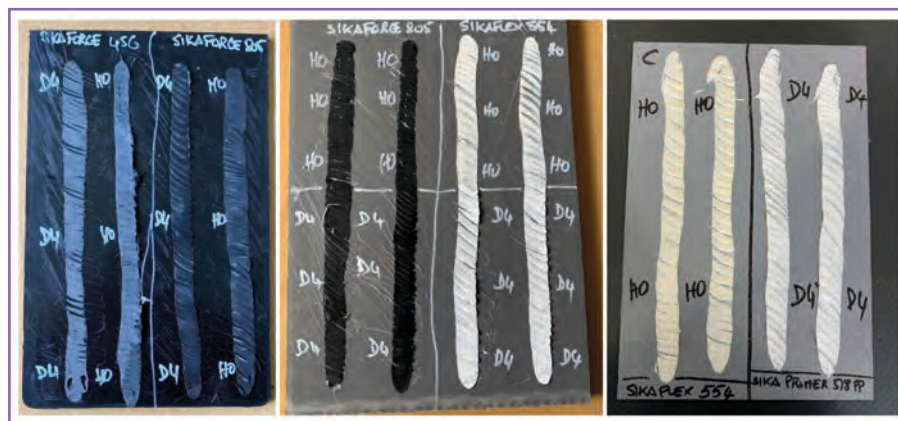
Fig. 4 - Adhesion peel test results on different PP materials with different adhesives after treatment with Sika® Primer-518 PP
