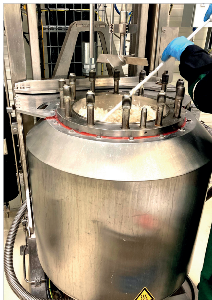
Fig. 2 - The process was scaled up at Fraunhofer CBP, where several kilograms of chicken feathers were processed. The process has been developed on a large scale at Fraunhofer CBP, treating several kilograms of chicken feathers.
